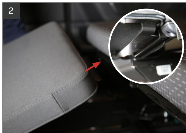
Fold-down the backrests and hook the bed extension into the bracket under the edge of the seat.
