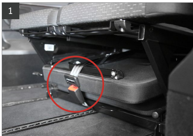
Open the safety belt buckle and take out both bed extension parts. The bed extension must be secured by the safety belt while driving!
